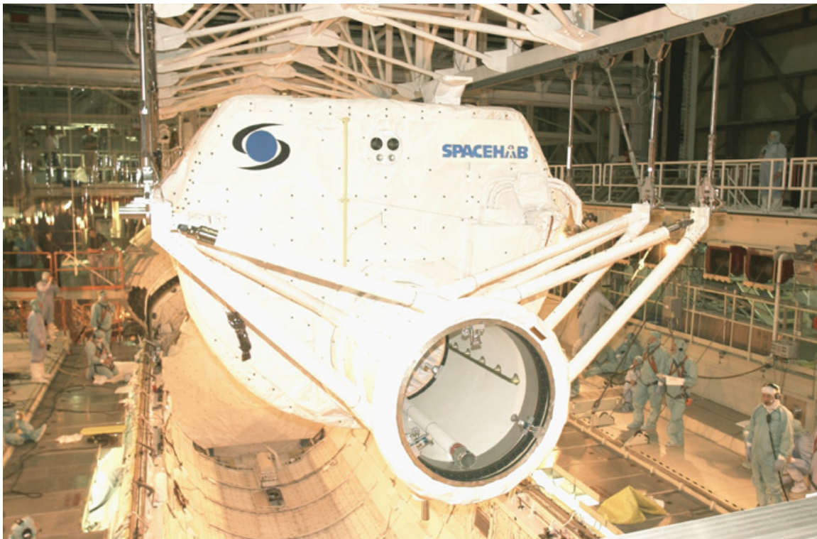
The SPACEHAB Research Double Module (RDM) and pressurized access tunnel are lowered toward Columbia's payload bay.
